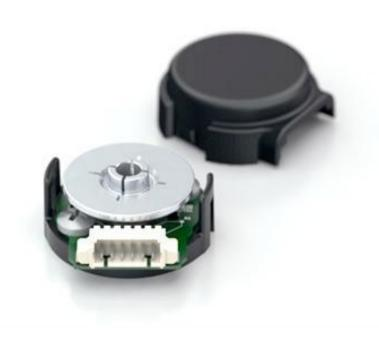
Converts angular position or motion of a shaft/axle to digital signal
